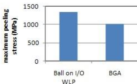
Figure 9 maximum peeling stresses for corner balls in U1 for scenario 2
